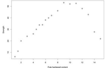
**Figure 11.5:** A Plot of Tensile Strength of Paper against the Percentage of Hardwood in the Pulp.
