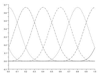
Fig. 13.5 Cubic B-spline based fuzzy partition
