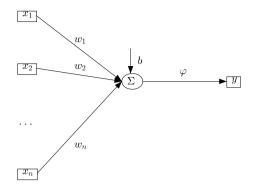
Fig. 14.1 The structure of an artificial neuron
