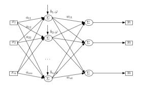
Fig. 14.4 The structure of a feed-forward neural network with multiple inputs and a single output
