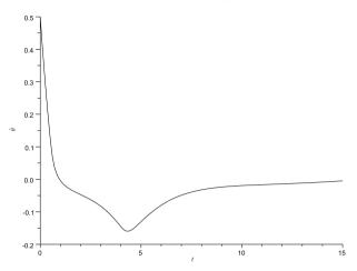
Fig. 7.10 The time dependence of the angular velocity  $\dot{\theta}$  for an inverted pendulum with a fuzzy controller
