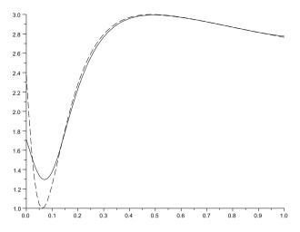
**Fig. 13.6** Approximation by cubic B-spline F-transform. Dashed line =  $f_1$ , solid line = inverse F-transform
