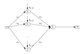
Fig. 14.2 The structure of a feed-forward neural network with a single input
