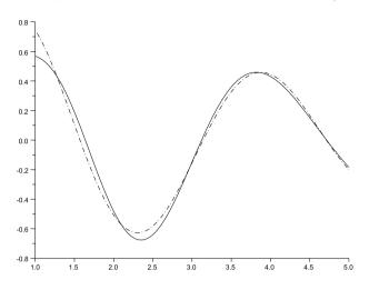
**Fig. 14.5** Approximation by a neural network. Dashed line  $f_1$  and solid line = neural network
