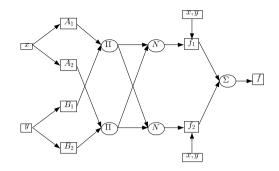
Fig. 14.7 The structure of a feedforward neural network with multiple inputs and a single output
