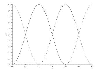
Fig. 13.3 Fuzzy Partition with trigonometric membership functions
