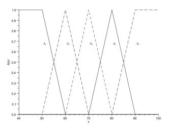
Fig. 1.4 Fuzzy sets Cold, Cool, Just Right, Warm and Hot used in a room temperature control example
