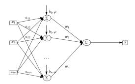
Fig. 14.3 The structure of a feed-forward neural network with multiple inputs and a single output
