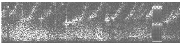
Figure 5. Example of Sonar Recording; Time is Horizontal Axis and Frequency is Vertical Axis
