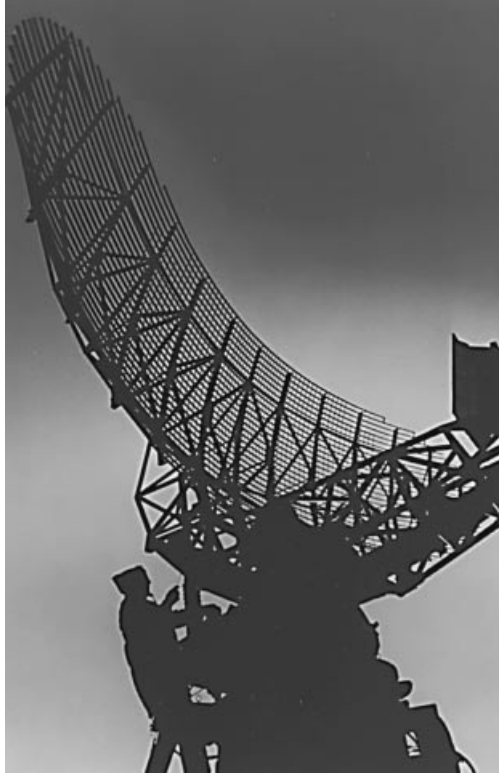
Figure 1.1-4 Fan-beam track-while-scan shipboard AN/SPS-49 radar [3]. Two hundred ten radars have been manufactured. (Photo courtesy of Raytheon Company.)
