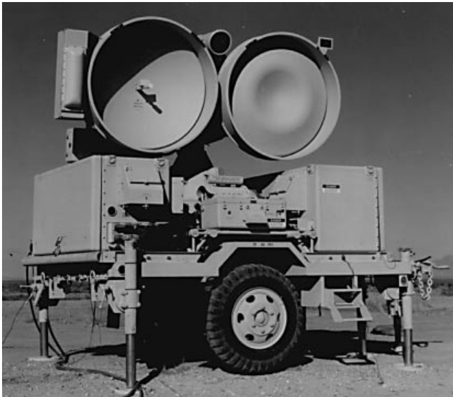
Figure 1.1-19 Hawk tracker-illuminator incorporating phase 3 product improvement kit, which consisted of improved digital computer and the Low Altitude Simultaneous HAWK Engagement (LASHE) antenna (small vertically oriented antenna to the left of main transmit antenna, which in turn is to the left of main receive antenna). Plans are underway to use this system with the AMRAAM missile. (Photo courtesy of Raytheon Company.)
