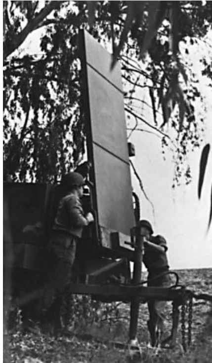
Figure 1.1-16 Short-range, limited-scan, electronically scanned (phase-frequency) phased-array artillery locating Firefinder AN/TPQ-36 radar [1]. Two hundred forty-three have been built. (Photo courtesy of Hughes Co.)
