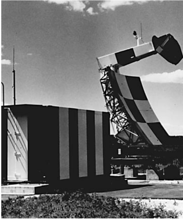
Figure 1.1-8 Limited-scan, electronically scanned phased-array AN/GPS-22 HiPAR. Used for guiding aircraft during landing under conditions of poor visibility [1–3]. Sixty systems deployed around the world [137]. (Photo courtesy of Raytheon Company.)
