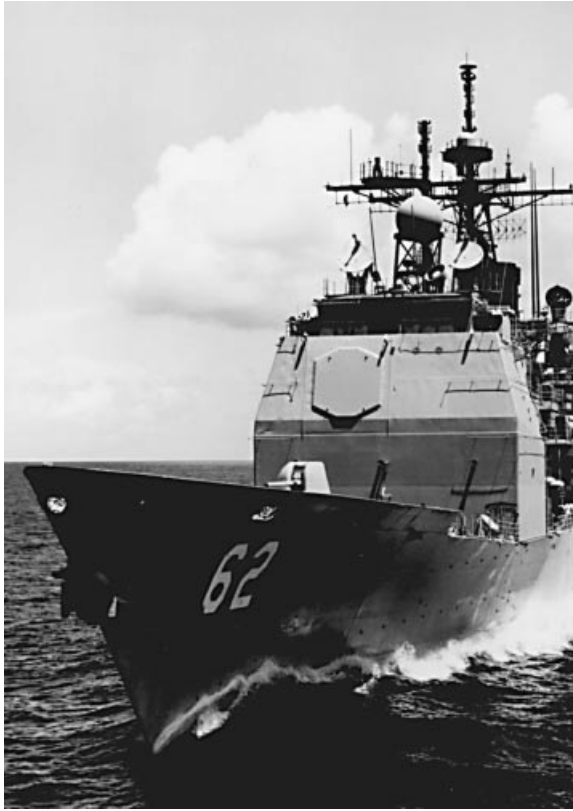
Figure 1.1-10 Multifunction shipboard AEGIS electronically scanned phased-array radar used to track many targets while also doing search on a time-shared basis. [1, 3]. Two hundred thirty-four array faces built each with about 4000 radiating elements and phase shifters [137]. (Photo courtesy of Raytheon Company.)
