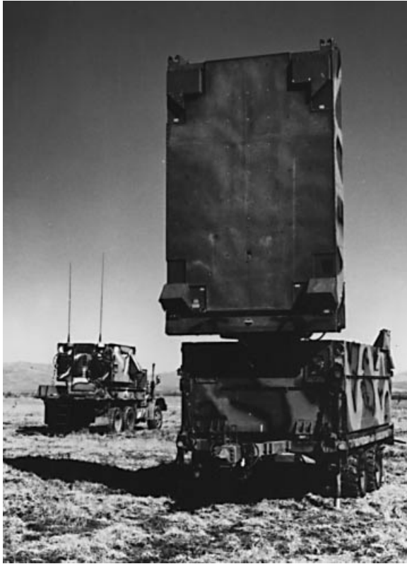
Figure 1.1-15 Long-range limited electronically scanned (phase-phase), phased-array artillery locating Firefinder AN/TPQ-37 radar [1]. One hundred two have been built and it is still in production [137]. (Photo courtesy of Hughes Aircraft.)
