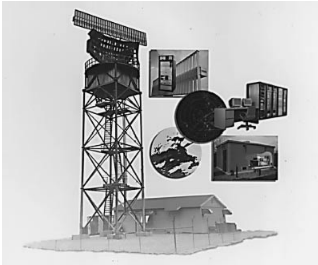
Figure 1.1-2 New combined Department of Defense (DOD) and Federal Aviation Administration (FAA) S Band fan-beam track-while-scan Digital Airport Surveillance Radar (DASR) ASR-11. This primary system uses a 17-kW peak-power solid-state “bottle” transmitter. Mounted on top of ASR-11 primary radar antenna is L-band open-array rectangular antenna of colocated Monopulse Secondary Surveillance Radar (MSSR). Up to 200 of these systems to be emplaced around the United States. (Photo courtesy of Raytheon Company.)
