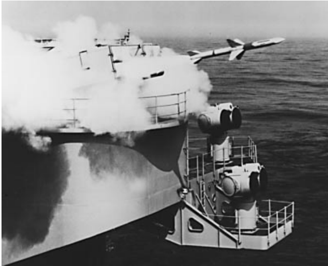
Figure 1.1-20 NATO SEASPARROW shipborne dedicated tracker-illuminator antenna [3]. One hundred twenty-three have been built. (Photo courtesy of Raytheon Company.)
